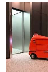
Coordination of elevator and delivery robot DeliRo (verification test at JR Meguro MARC Building)
