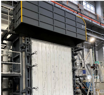
Exterior wall fireproof test (product development)
