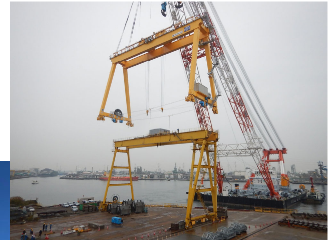
Gantry crane delivered by floating crane (FC)
