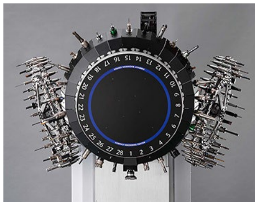
Newly developed 100-tool magazine
