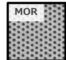
**MOR (Metal Oxide Resist)** ◎ Sensitivity and etching resistance
