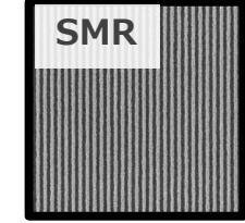
**SMR (Small Molecular Resist)** ◎ Pattern uniformity and etching resistance
