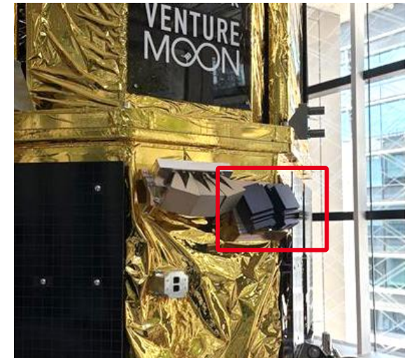
In the above photo, the red frame shows the LRF. It is installed on the side of the lander.
