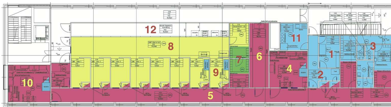
1, 2 & 11 = Material Flow Intake Rooms 4 = Preparation Room (Grade D) 6 = Cell Culture Material Storage (Grade D) 8 = Incubators & Refrigerators (Grade B) 10 = Freezing & Storage Room (Grade D) 3 = Gowning/De-gowning Rooms 5 = Supply Corridor (Grade D) 7 = Passage to Grade B Section (Grade C) 9 = Working Units (Grade B) 12 = Maintenance Corridor
