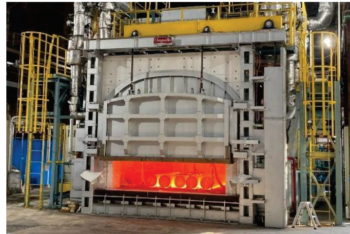
The demonstration furnace employs a hydrogen burner capable of firing 100% hydrogen, a hydrogen/city gas blend, or 100% city gas.
