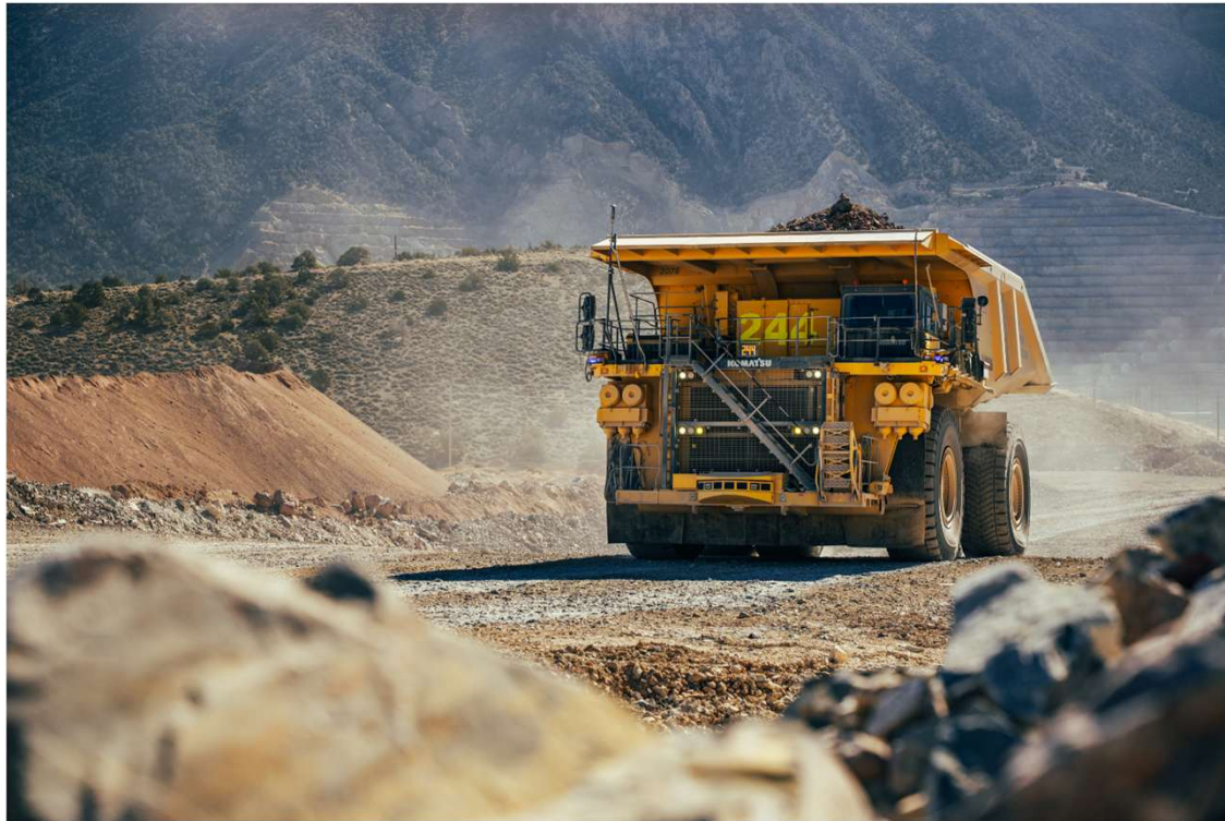
A 930E-5AT AHS haul truck in operation at Nevada Gold Mines, U.S.
