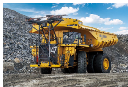
[Diesel trolley Power Agnostic 930E truck operating at the Boliden copper mine]
