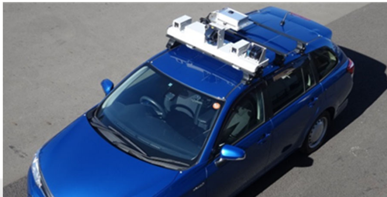
Road Surface Properties Measuring Vehicle
