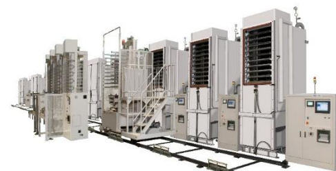
Vacuum Hot Press Machine for High-Multilayer PCB
