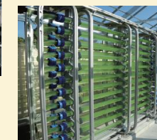
Microalgae cultivation facility (sealed glass tubes type photobioreactor)
