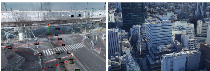
Measurement views in 3Dmapspocket® (left: high-precision 3D point cloud data; right: Google Photorealistic 3D Tiles)
