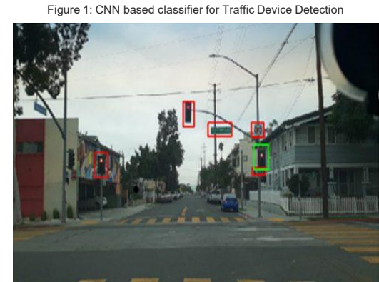
Figure 1: CNN based classifier for Traffic Device Detection
