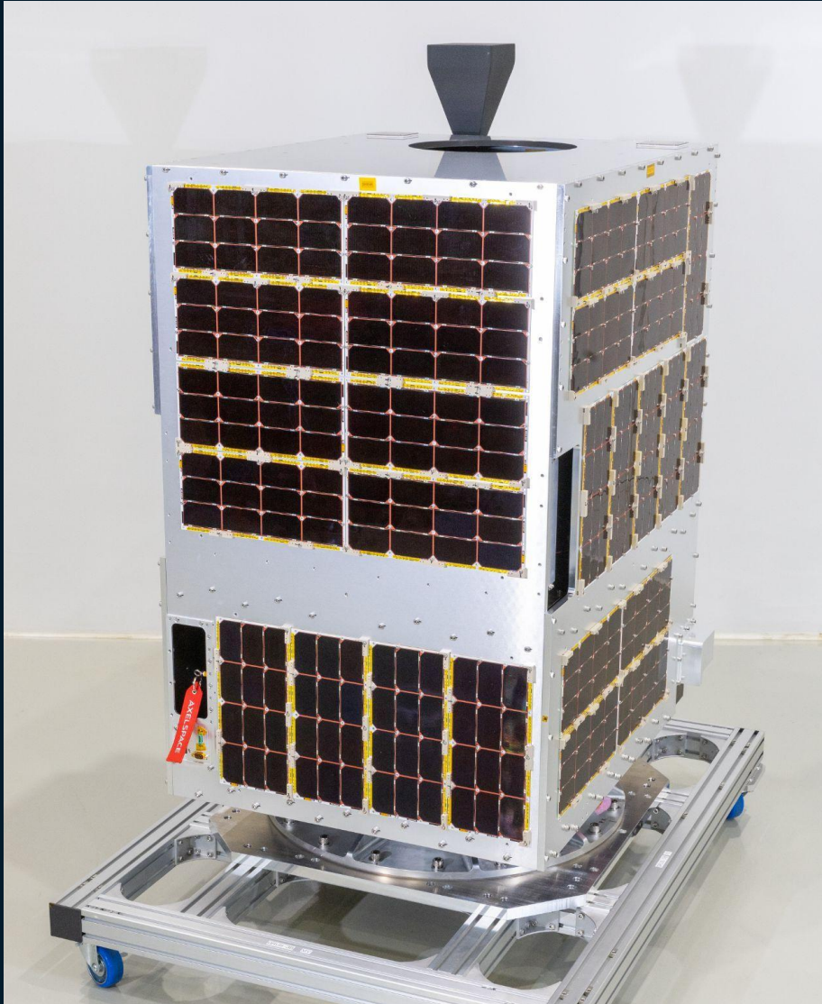
Flight Model of GRUS-3
