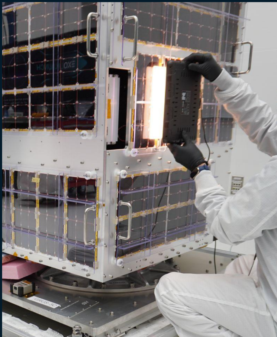
Solar panel health testing for GRUS-3
